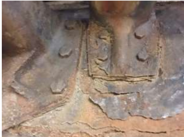
Undercarriage and frame corrosion on E7 after only 12 years of service
