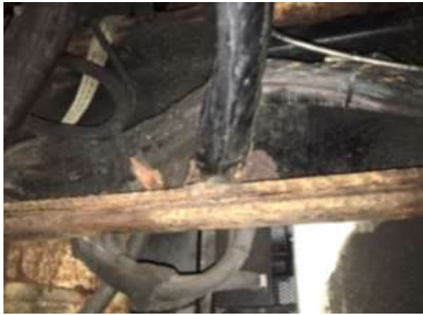
Undercarriage and frame corrosion on E7 after only 12 years of service
