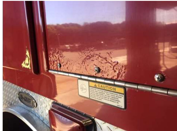
Exterior paint corrosion on doors and compartments caused by road chemicals
