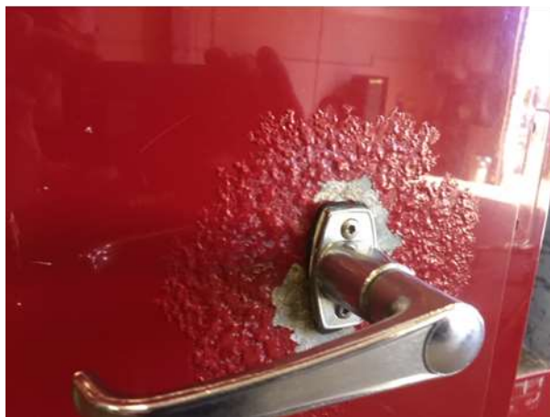
Exterior paint corrosion on doors and compartments caused by road chemicals
